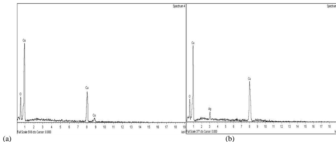
**Fig.1.** EDS spectra (a) pure and (b) Ag(4at.%) doped Cu<sub>2</sub>O films.
