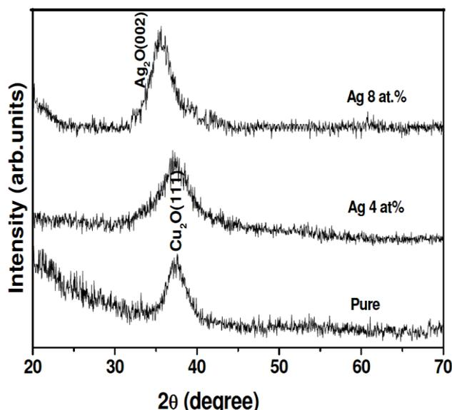
Fig.2. XRD patterns of pure and Ag doped  $\text{Cu}_2\text{O}$  films.
