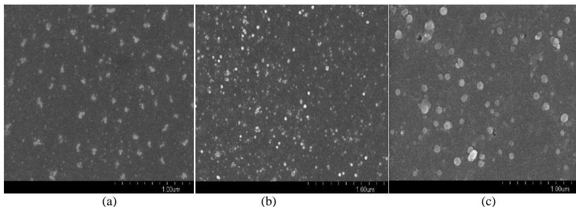
**Fig.3.** SEM images: (a) pure, (b) Ag(4at.%) $\text{-Cu}_2\text{O}$  and (c) Ag(8at.%) $\text{-Cu}_2\text{O}$  films.
